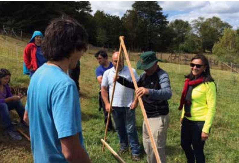
Teaching students how to use the A frame to mark contours on a hill side in Chiloe, Chile. Photo: Clara Nicholls
